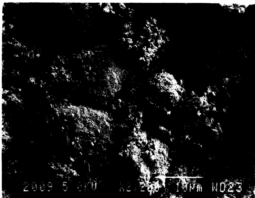
Fig. 5. (b) SEM of the heated mechanical mixture of silver oxalate and nickel oxalate (2a) up to 500°C.
